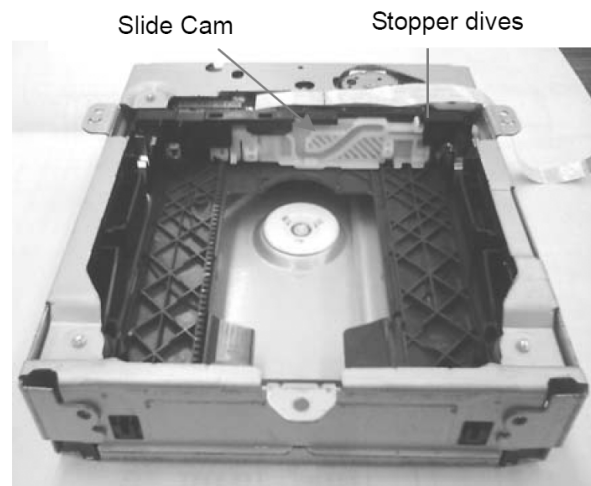
After fall down of Traverse Base
